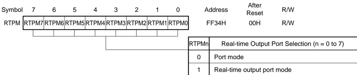
**Cautions** 1. When using these bits as a real-time output port, set the ports to which real-time output is performed to the output mode (clear the corresponding bit of the port mode register 12 (PM12) to 0).
