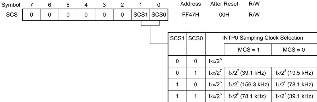
**Caution**  $f_{xx}/2^N$  is the clock supplied to the CPU, and  $f_{xx}/2^5$ ,  $f_{xx}/2^6$ , and  $f_{xx}/2^7$  are clocks supplied to peripheral hardware. The  $f_{xx}/2^N$  clock is stopped in HALT mode.
