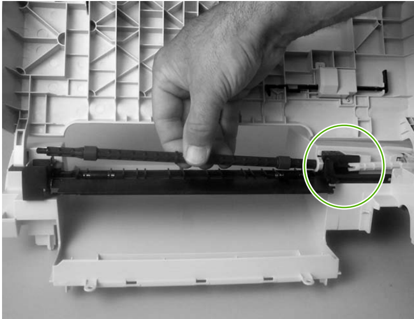
Figure 5-36 Remove the duplex-reverse-drive assembly (2 of 5)
