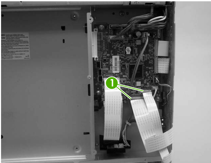
Figure 5-88 Remove the high-voltage power supply (1 of 3)
