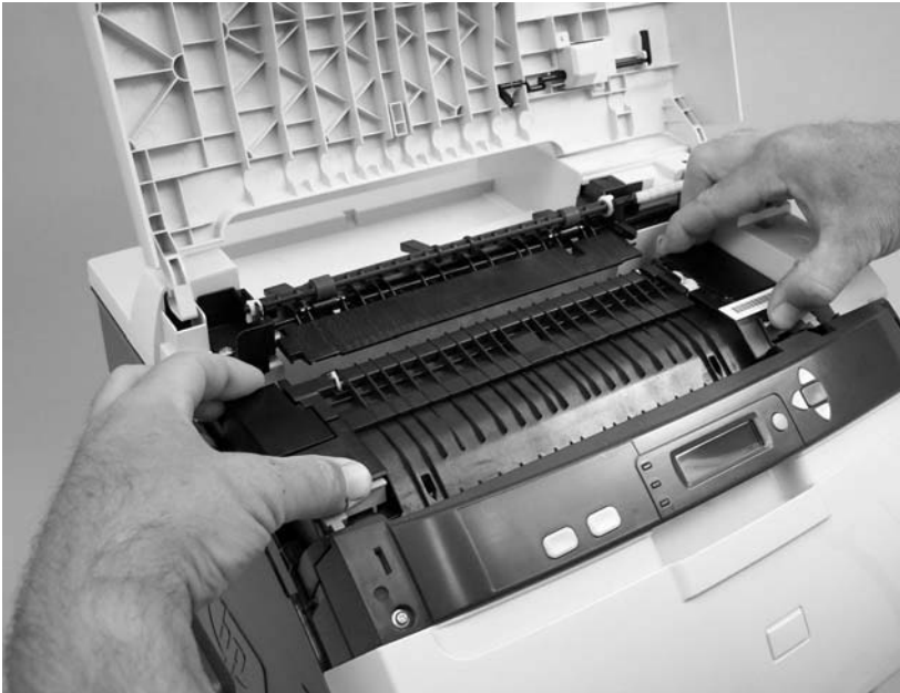
Figure 5-12 Remove the upper cover (2 of 5)
