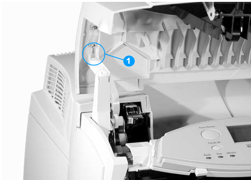
Figure 6-3 Removing and replacing the top cover (1 of 2)
