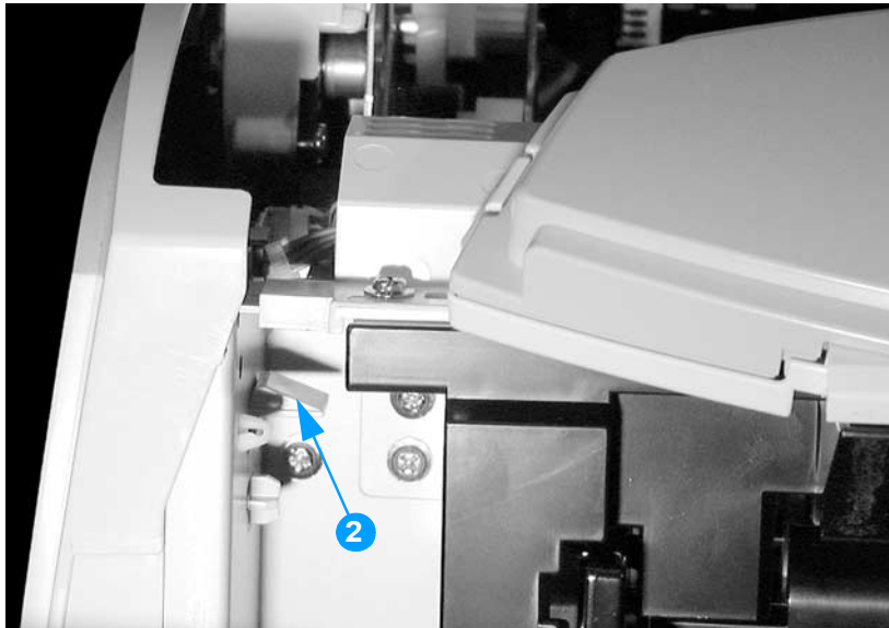
Figure 6-9 Removing and replacing the left cover (2 of 2)
