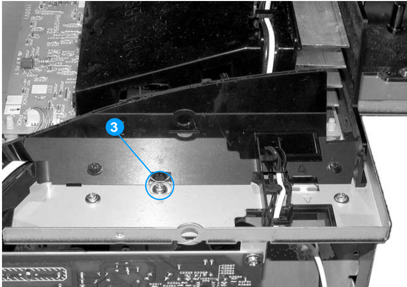
Figure 6-54 Removing and replacing the right side laser/scanner retaining bar, right side of printer (1 of 2)
