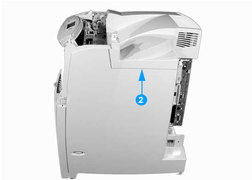
Figure 6-6 Removing and replacing the rear top cover, releasing right-side tab (2 of 3)
