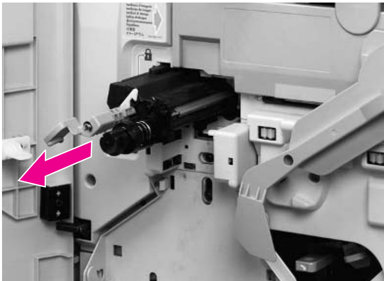
Figure 79. Remove the transfer cleaner
