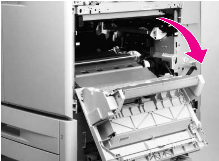
Figure 103. Open the ITB door
