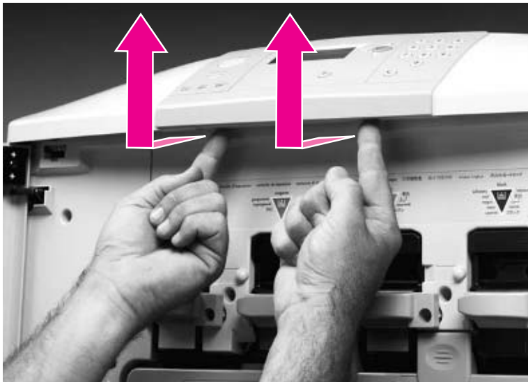
Figure 83. Release the control panel
