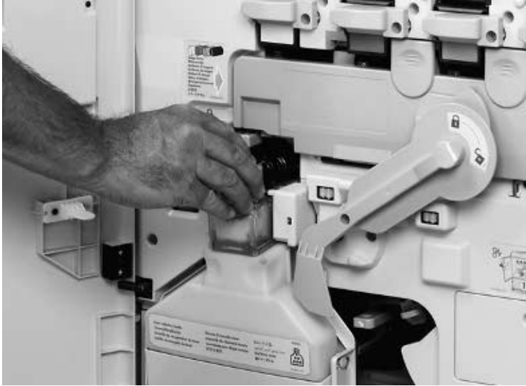
Figure 77. Remove the waste toner bottle
