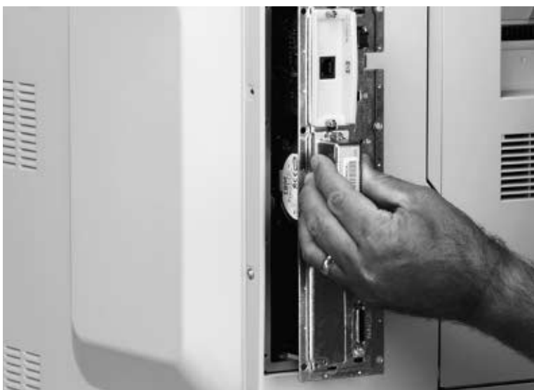
Figure 230. Remove the formatter PCB
