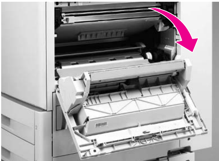
Figure 160. Open the ITB door
