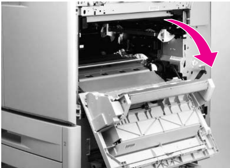
Figure 182. Open the ITB door
