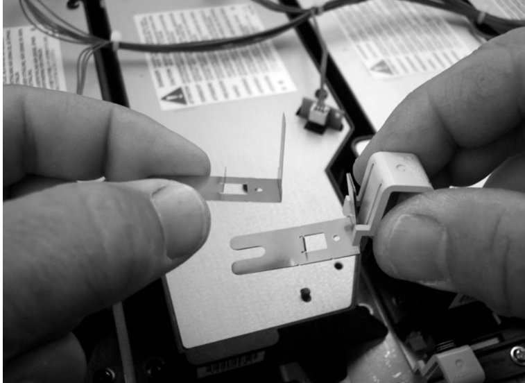
Figure 136. Add or remove the laser/scanner adjustment shims
