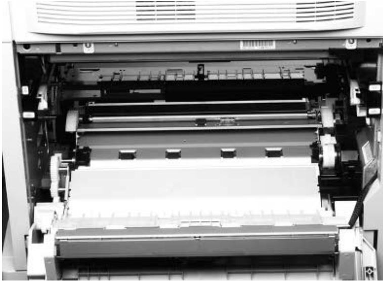
Figure 178. Remove the T2 assembly
