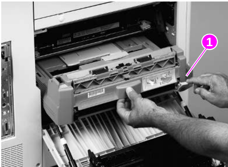
Figure 156. Remove the duplexer
