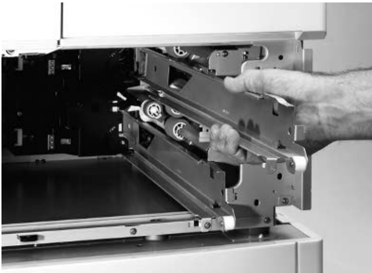
Figure 192. Remove the tray guides
