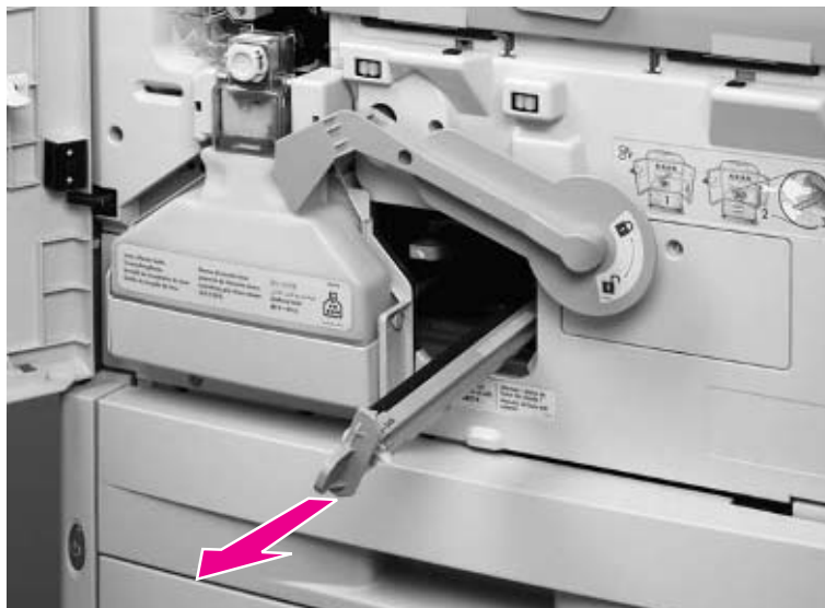
Figure 81. Remove the transfer roller
