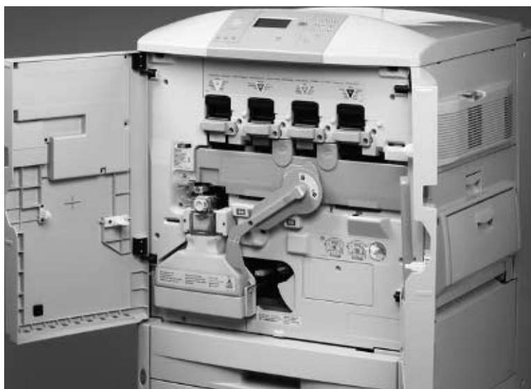
Figure 203. Gain access to the green ITB release lever
