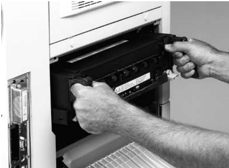
Figure 158. Remove the fuser
