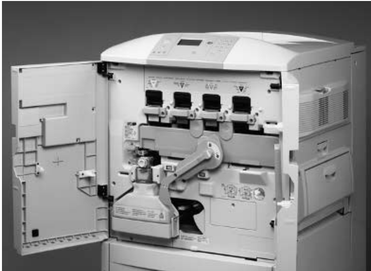
Figure 70. Gain access to the toner cartridges
