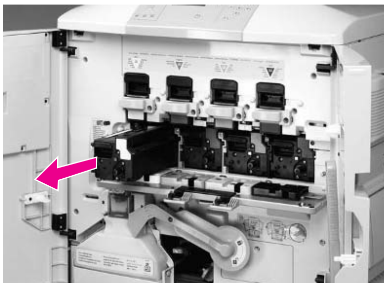
Figure 76. Remove the process cartridges
