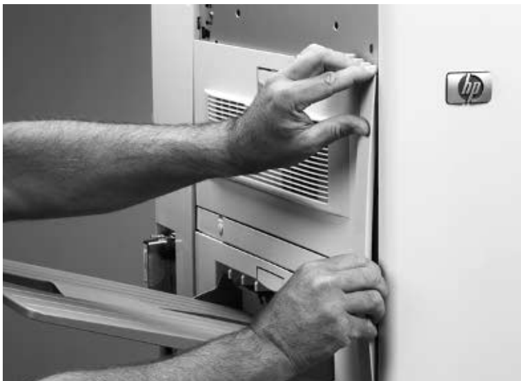
Figure 141. Remove the left side front cover
