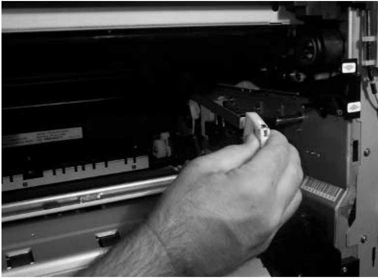
Figure 206. Remove the right back ITB lifting link
