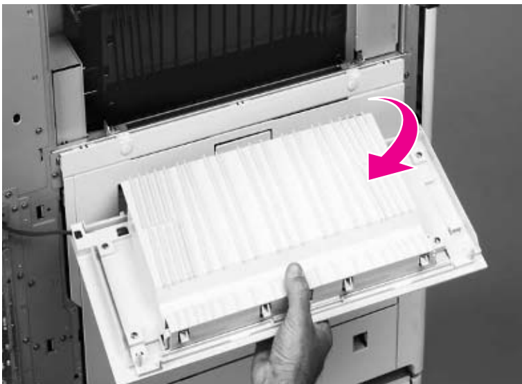
Figure 149. Remove the paper path access door
