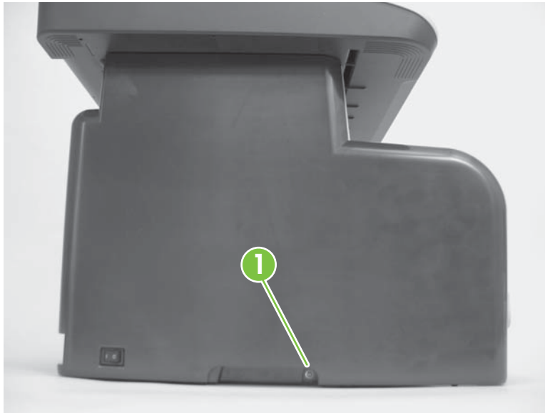
Figure 6-40 Remove the left cover (1 of 4)
