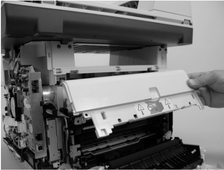
Figure 6-54 Remove the rear-upper cover (2 of 2)
