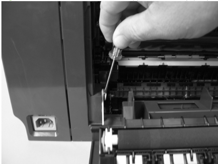
Figure 6-31 Remove the rear-door stopper and link cap (simplex product) (2 of 2)
