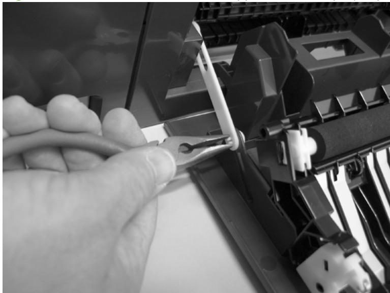
Figure 6-30 Remove the rear-door stopper and link caps (simplex product) (1 of 2)
