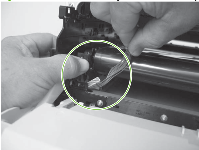
Figure 6-87 Reinstall the color-misregistration sensor assembly PCA (1 of 2)
