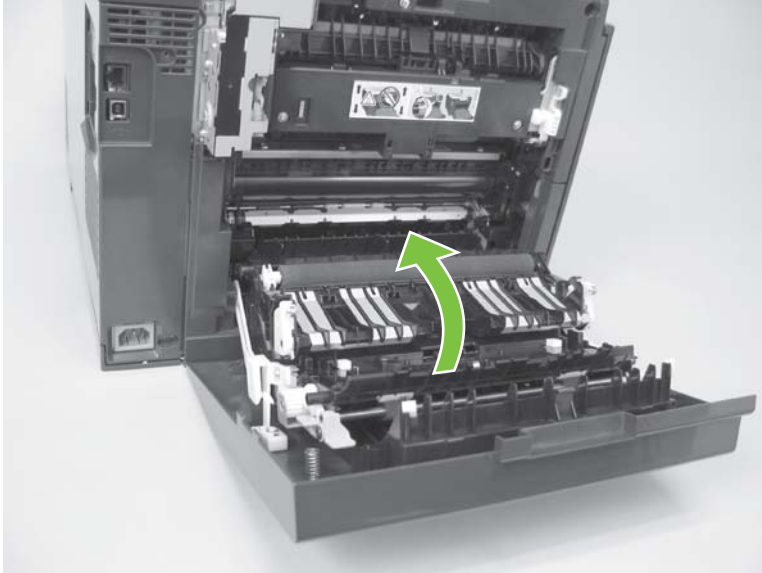
Figure 6-36 Remove the rear door (duplex product) (1 of 4)
