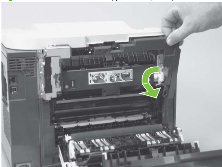
Figure 6-47 Remove the rear-upper cover (2 of 2)
