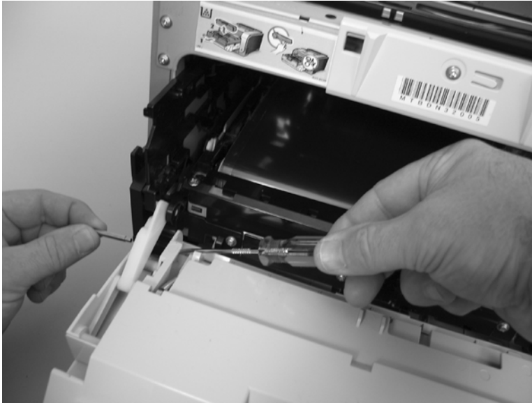
Figure 6-143 Remove the front-door assembly (2 of 10)
