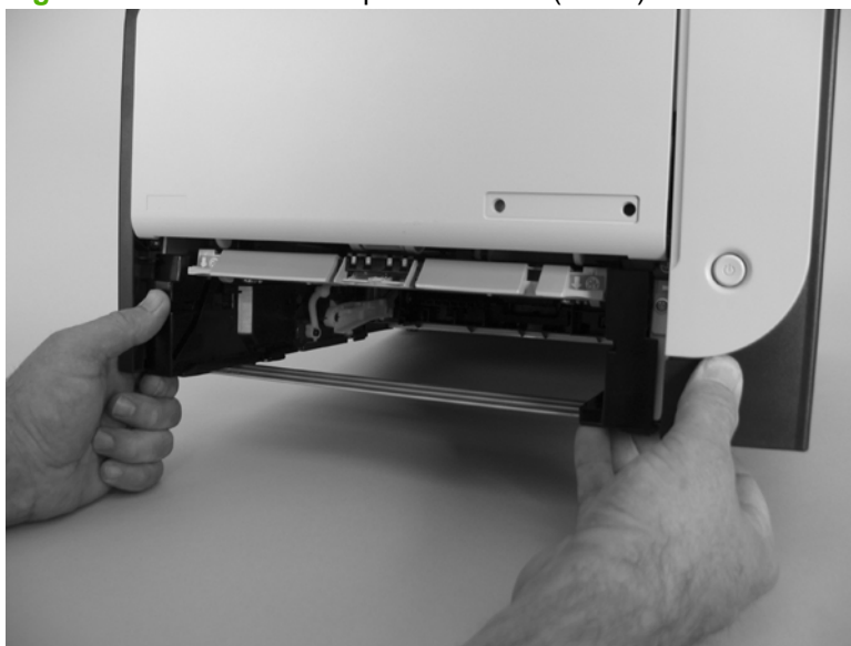
Figure 6-6 Remove the separation roller (1 of 3)
