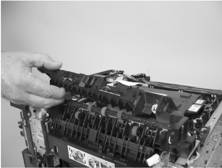
Figure 6-141 Remove the paper-delivery assembly (4 of 4)
