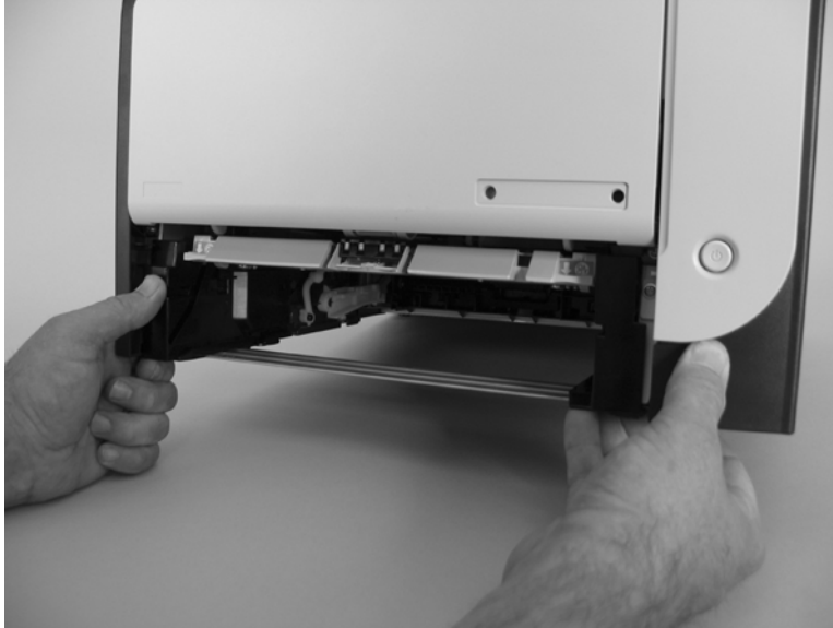
Figure 6-11 Remove the Tray 1 paper-pickup roller (2 of 3)
