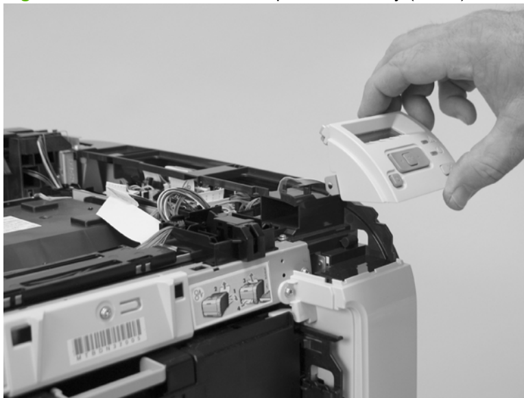
Figure 6-71 Remove the control-panel assembly (3 of 3)
