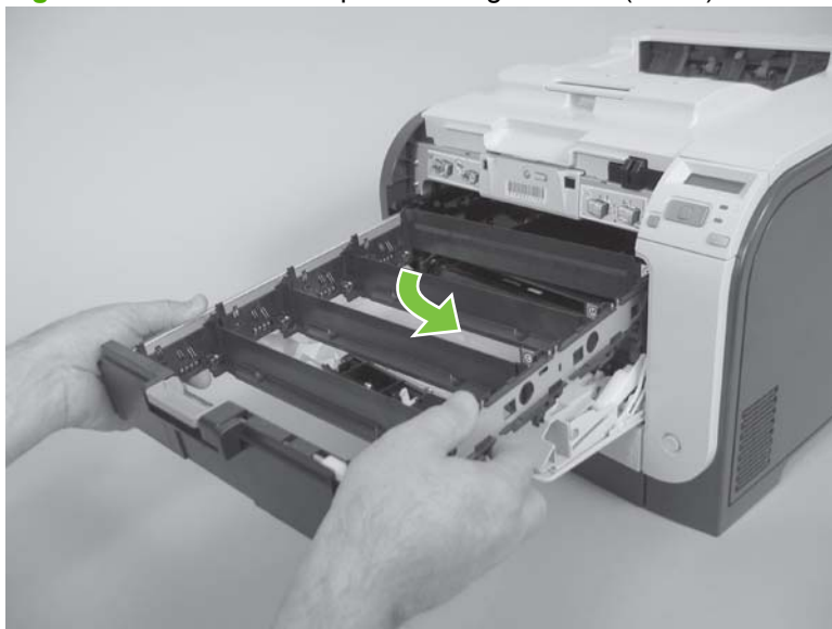
Figure 6-19 Remove the print-cartridge drawer (2 of 3)
