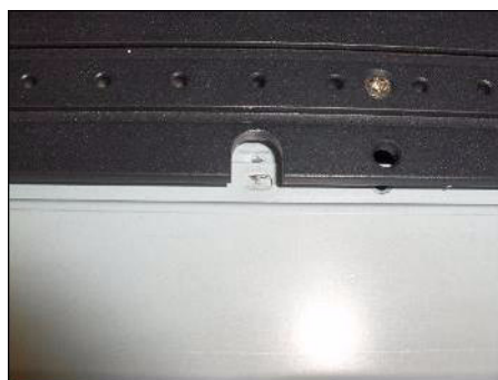
Correct insertion of the heater into the support slot
