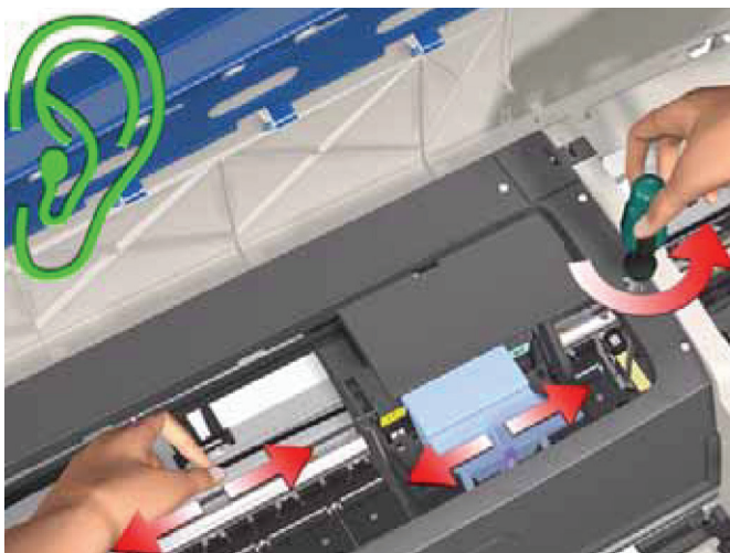
Figure 5-4 Cross-Section - Raising the Pivot Assembly
