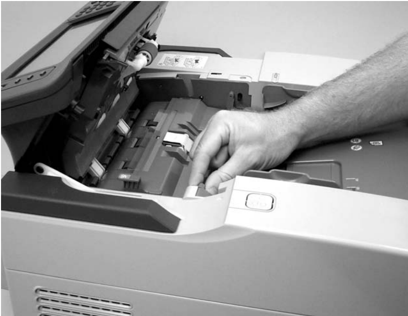
Figure 6-24 Removing the paper input tray
