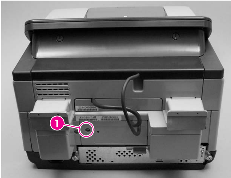
Figure 6-46 Removing the scanner rear cover
