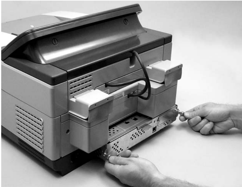
Figure 6-17 Removing the formatter cage
