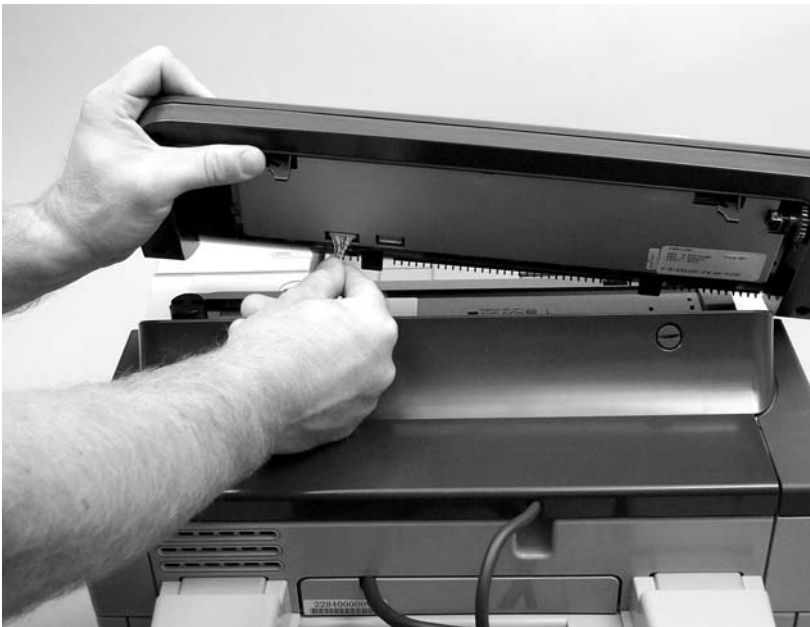
Figure 6-15 Removing the control panel (2 of 2)
