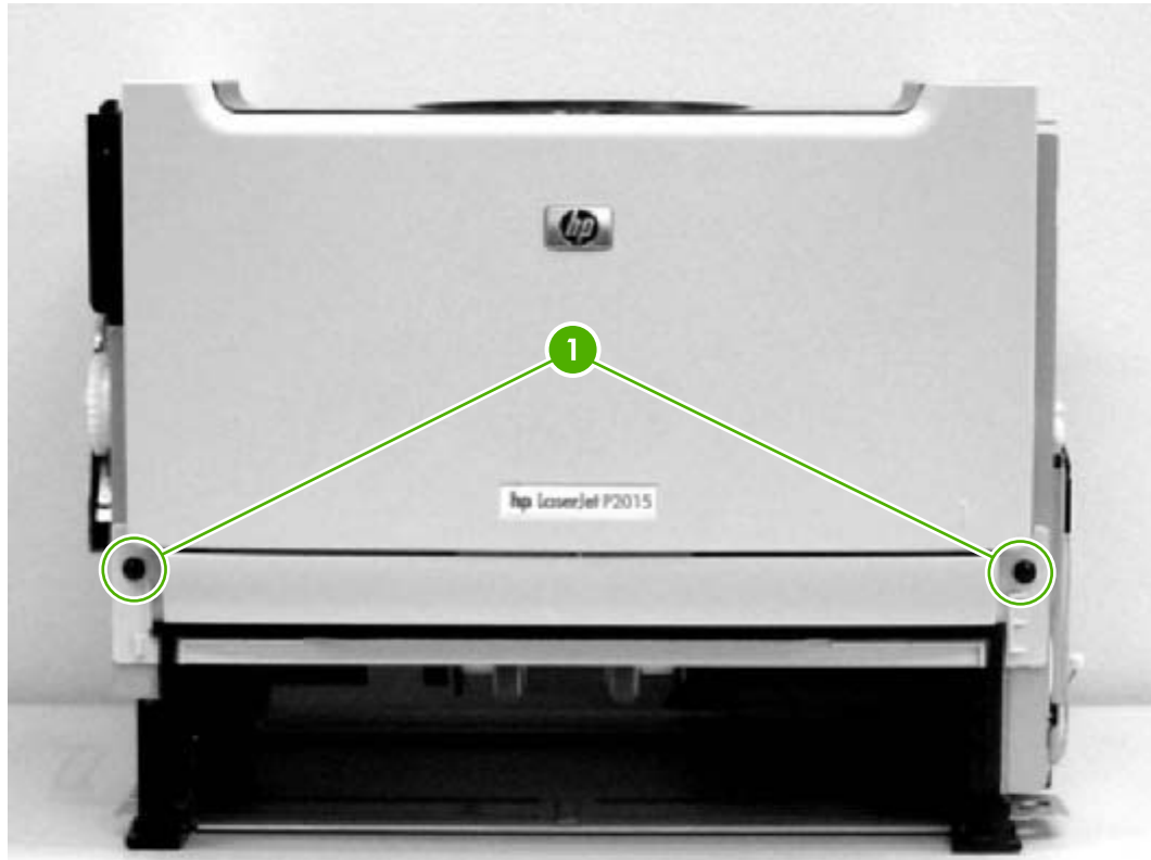
Figure 6-50 Removing the print-cartridge door (2 of 2)
