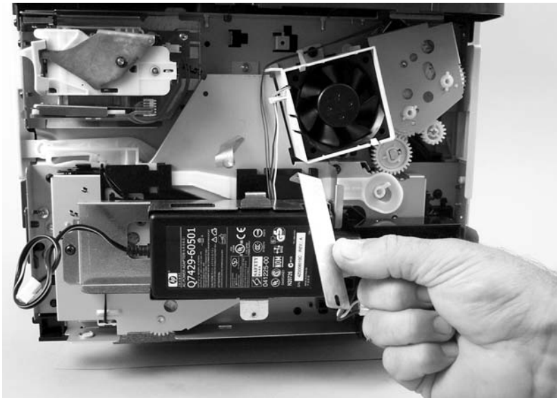
Figure 5-45 Remove the convenience-stapler power assembly (2 of 3)
