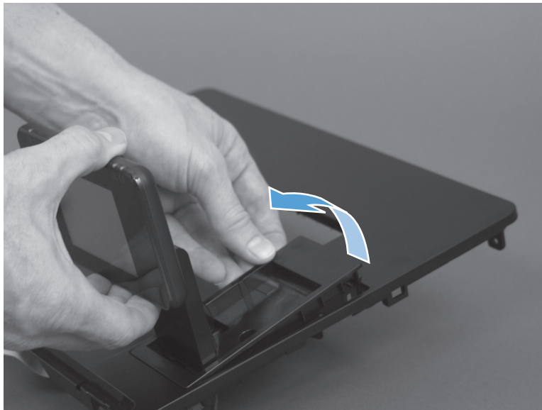
Figure 1-24 Remove the touchscreen control panel (3 of 3)
