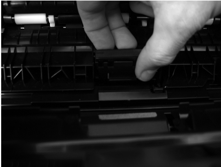
Figure 1-8 Remove the MP tray separation pad (5 of 5)
