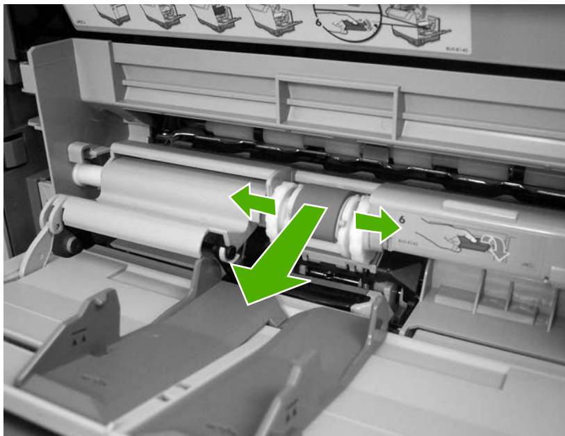
Figure 5-24 Remove the tray 1 pickup roller
