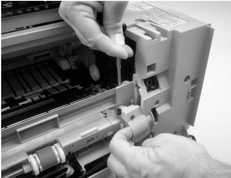
Figure 5-87 Remove the tray 1 feed-assembly (5 of 13)
