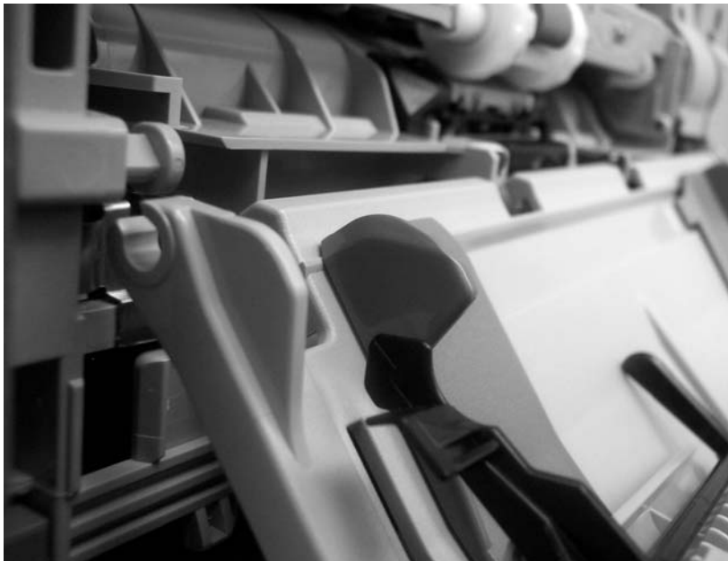
Figure 5-78 Remove the tray 1 assembly (4 of 5)
