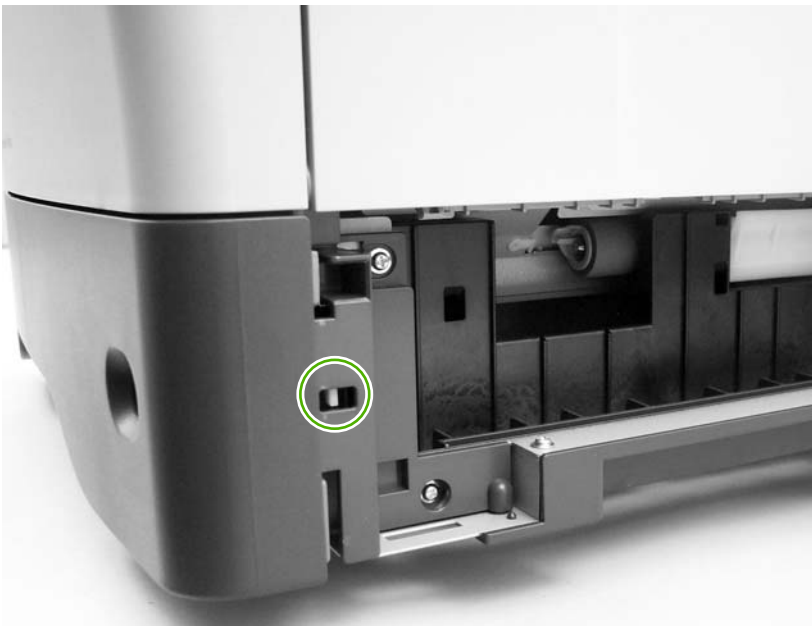
Figure 4-76 Tray 2 jam-access-cover switch, SW105
