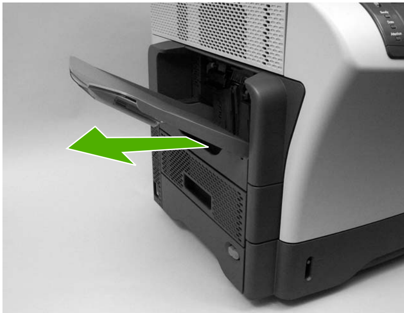
Figure 5-16 Remove the output-bin assembly (1 of 2)
