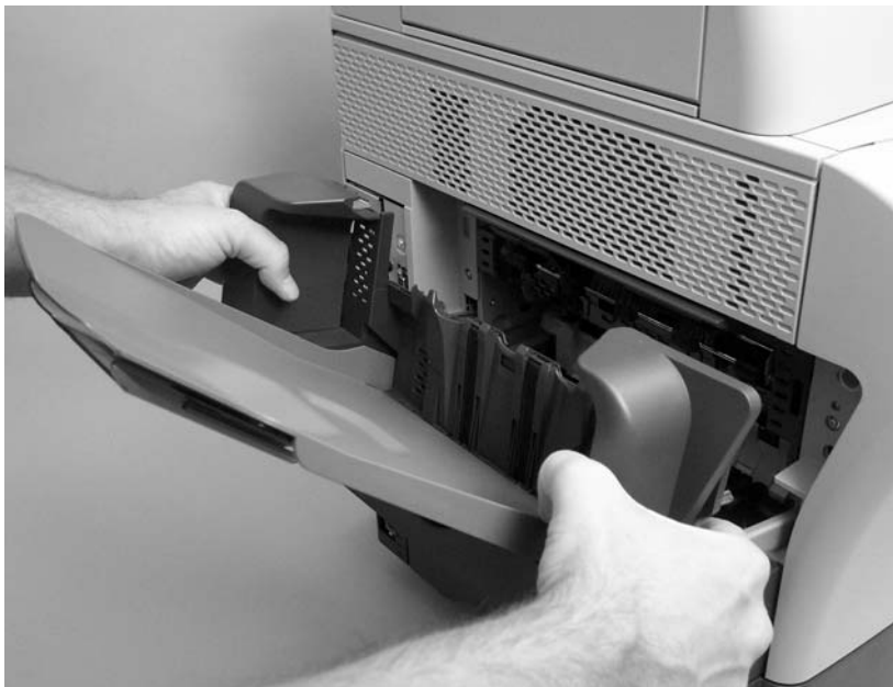
Figure 5-17 Remove the output-bin assembly (2 of 2)
