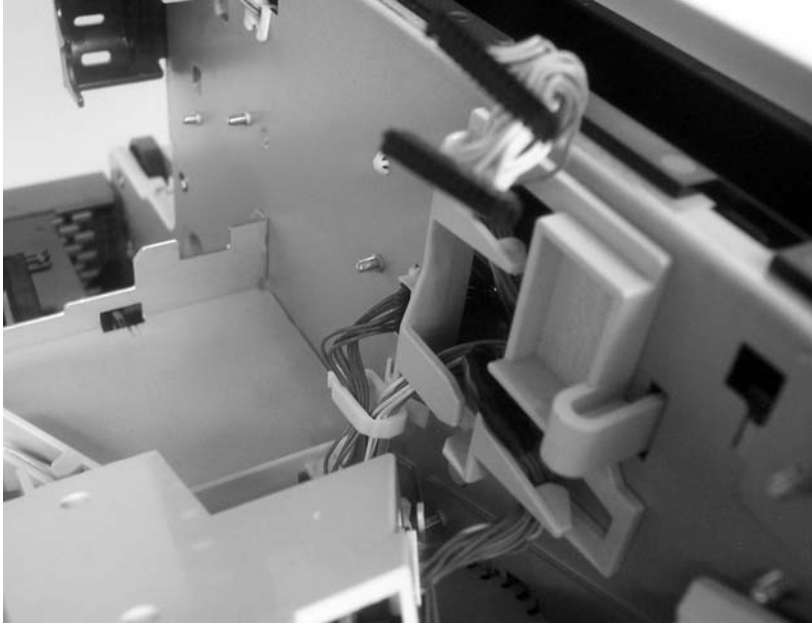
Figure 5-164 Remove the laser/scanner (1 of 2)
