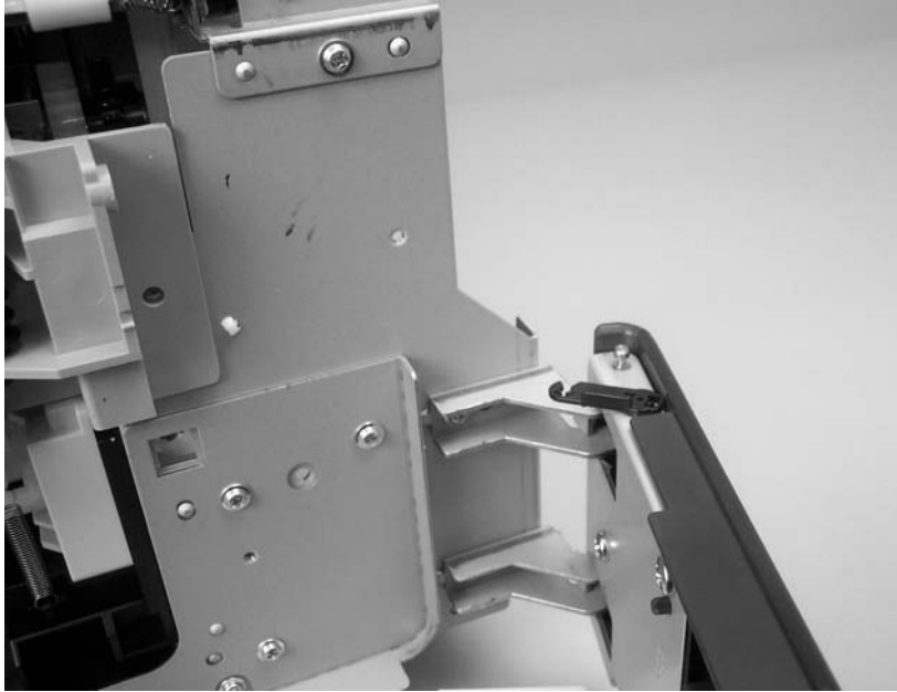
Figure 5-83 Remove the tray 1 feed-assembly (1 of 13)
