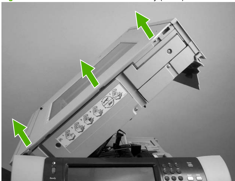
Figure 5-171 Remove the scanner assembly (1 of 8)
