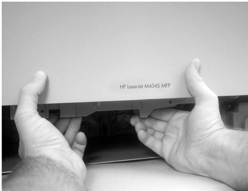
Figure 5-44 Remove the front cover (6 of 7)
