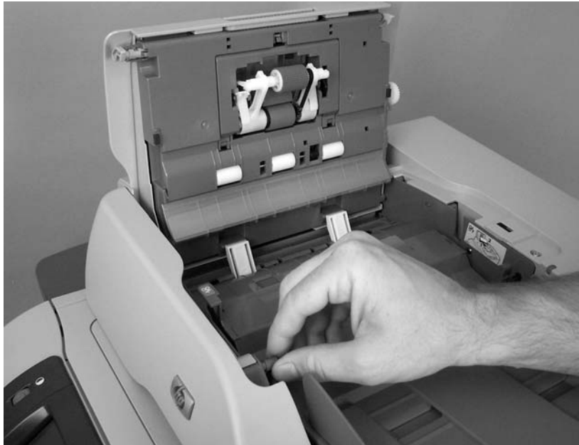
Figure 5-6 Remove the ADF input tray (2 of 3)
