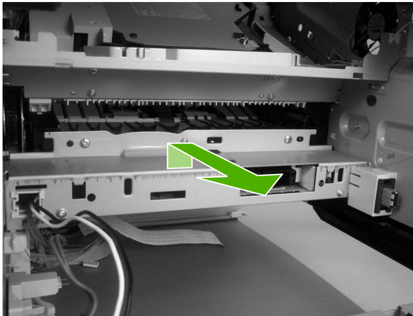
Figure 5-157 Remove the engine power supply (10 of 10)
