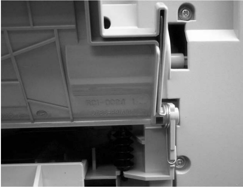
Figure 5-79 Correct tray 1 rear-hinge-spring placement
