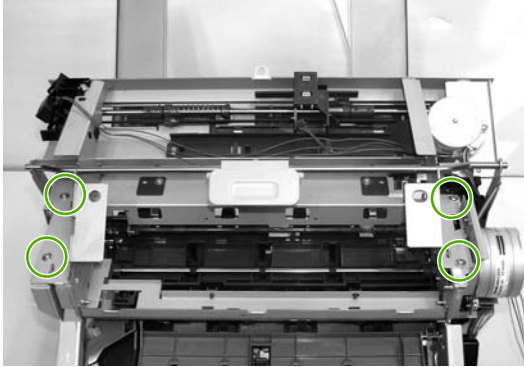
Figure 5-215 Remove the jogger unit (6 of 7)
