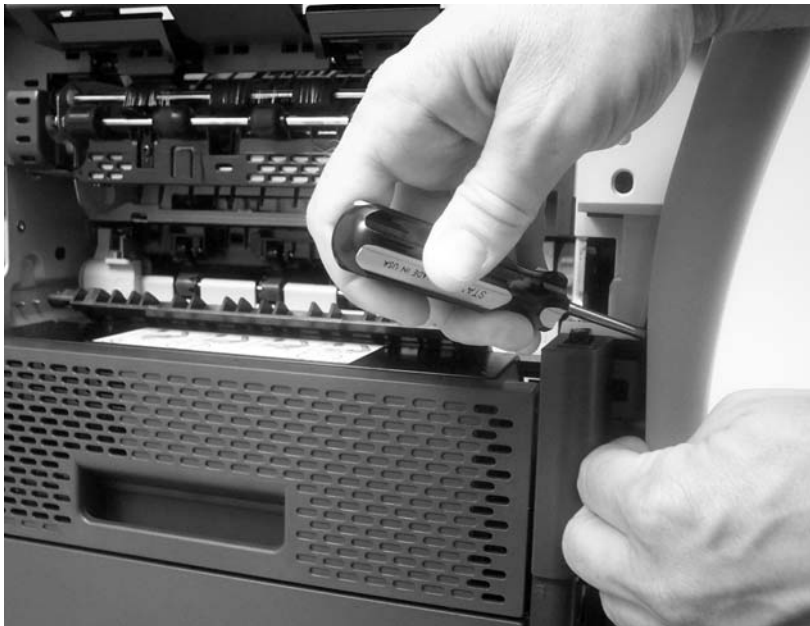
Figure 5-42 Remove the front cover (4 of 7)
