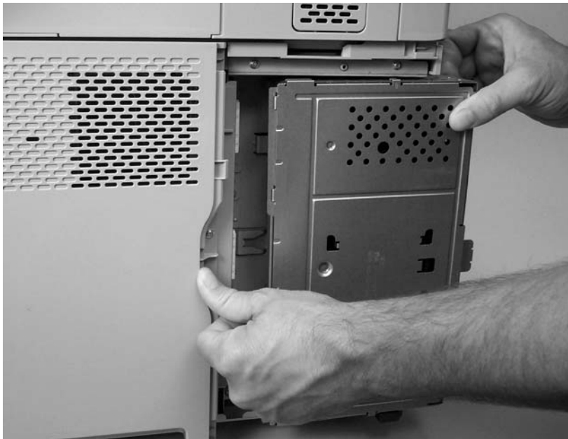
Figure 5-32 Remove the formatter cover and formatter (3 of 3)
