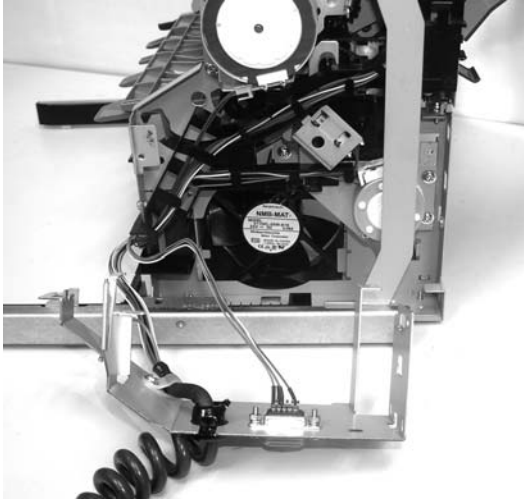
Figure 5-212 Remove the jogger unit (3 of 7)
