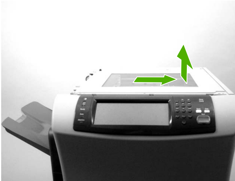
Figure 5-178 Remove the scanner assembly (8 of 8)
