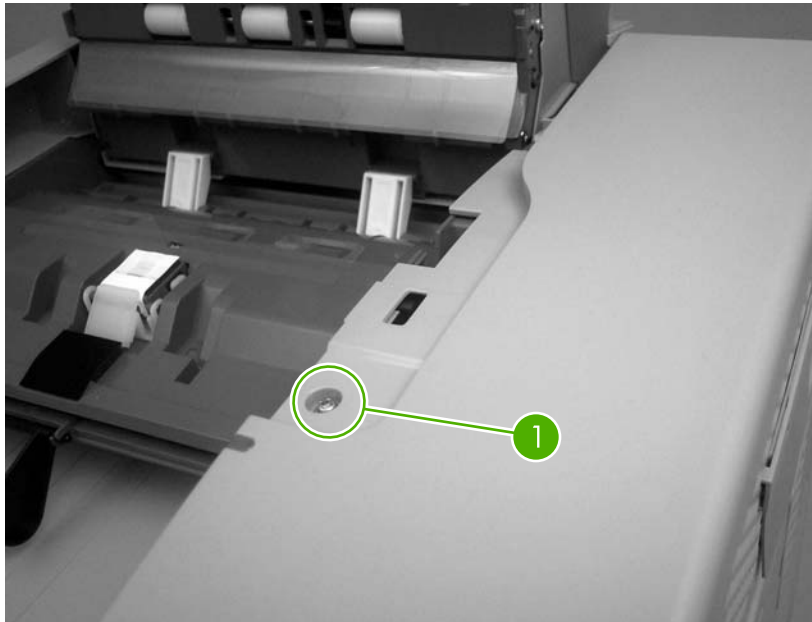
Figure 5-190 Remove the ADF rear cover (1 of 2)
