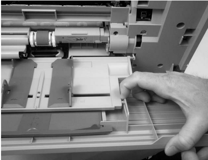
Figure 5-75 Remove the tray 1 assembly (1 of 5)
