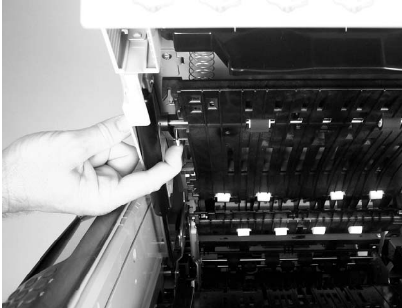
Figure 5-49 Remove the reversing-separation-guide assembly (1 of 2)
