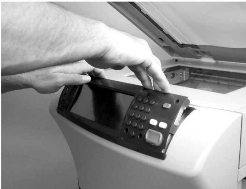
Figure 5-2 Remove the control panel (1 of 2)
