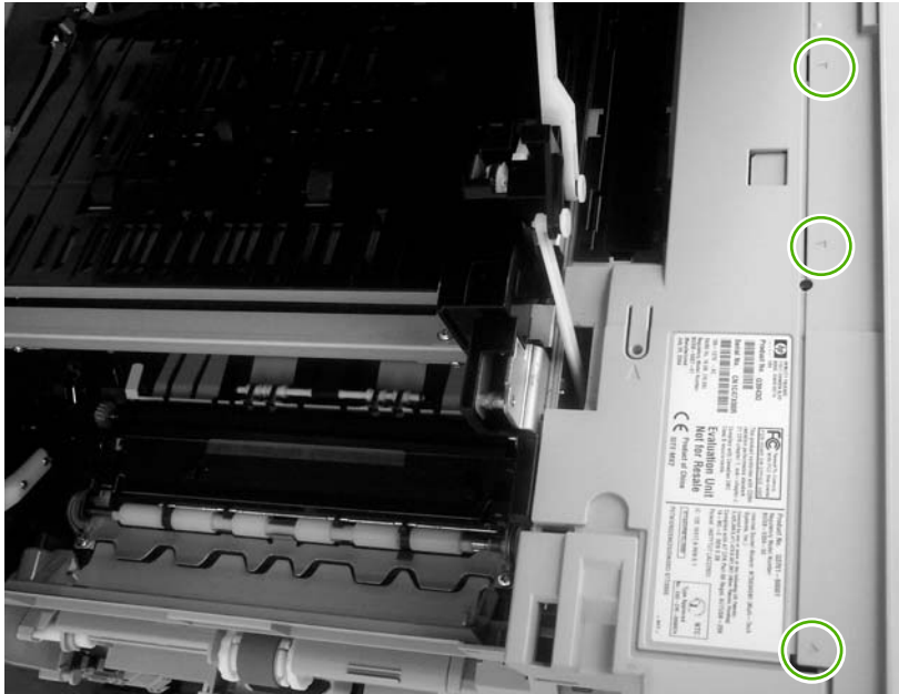
Figure 5-47 Remove the back cover (2 of 3)
