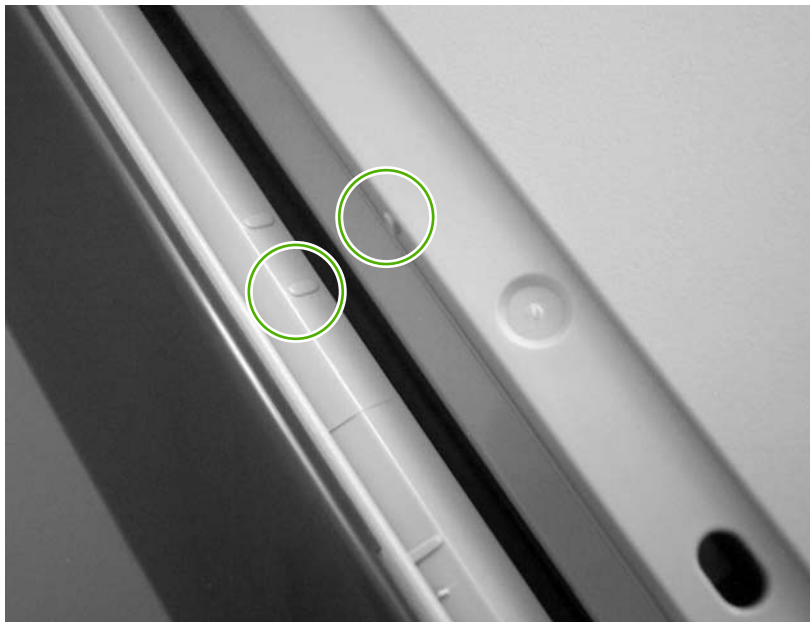
Figure 5-179 Correctly positioning the scanner assembly
