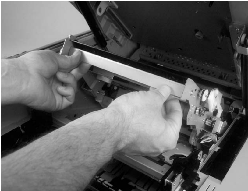
Figure 5-58 Remove the reversing assembly (8 of 8)
