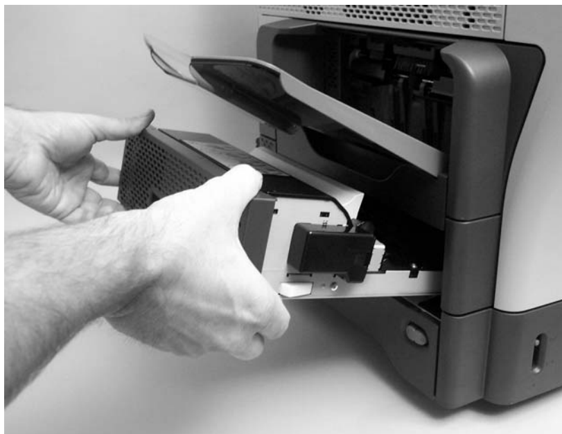
Figure 5-19 Remove the duplex-printing unit (2 of 2)
