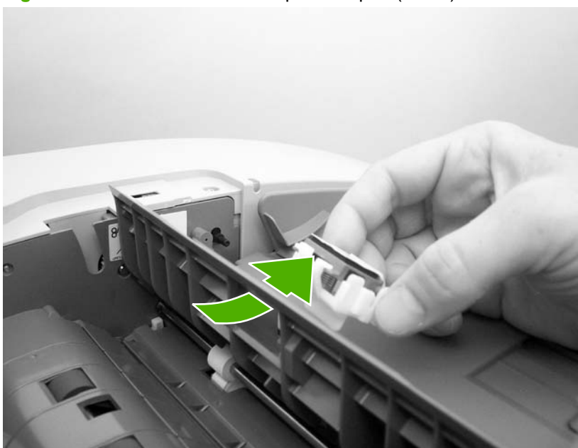
Figure 5-11 Remove the ADF separation pad (2 of 2)
