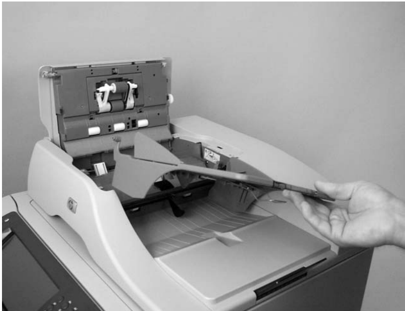
Figure 5-7 Remove the ADF input tray (3 of 3)
