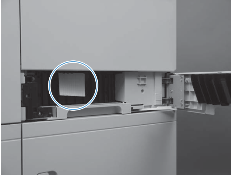
Figure 3-9 Test the PS102 pre-feed sensor
