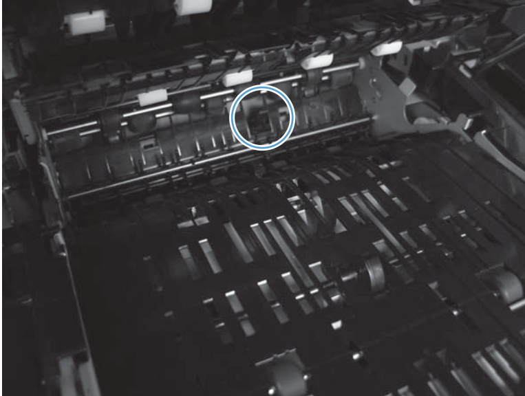
Figure 3-15 Test the PS112 output sensor
