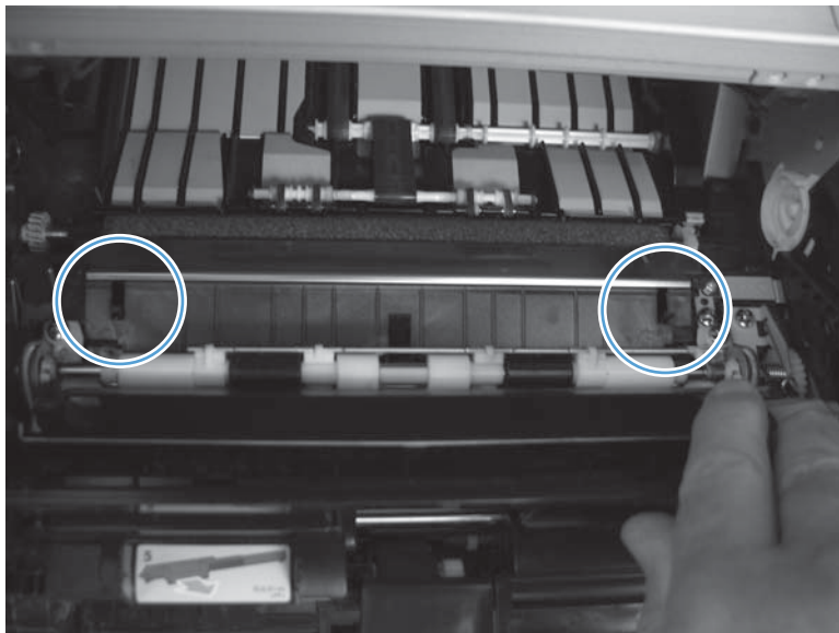
Figure 3-11 Test the PS106/108 paper width sensors
