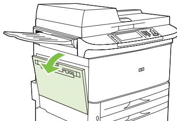
Figure 7-78 Clear jams in the left door (2 of 4)
