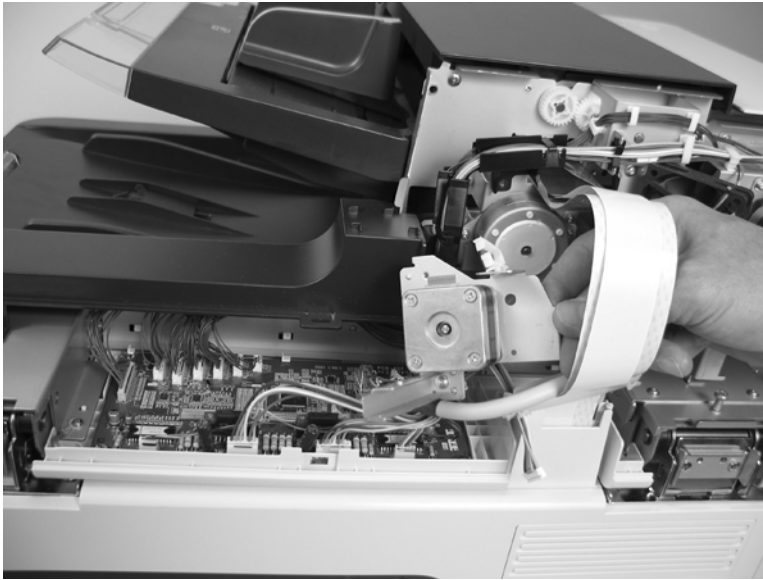
Figure 5-94 Remove the ADF exit-motor assembly (5 of 7)
