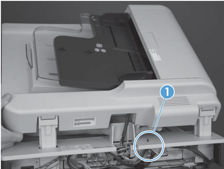
Figure 1-109 Remove the document feeder (3 of 4)
