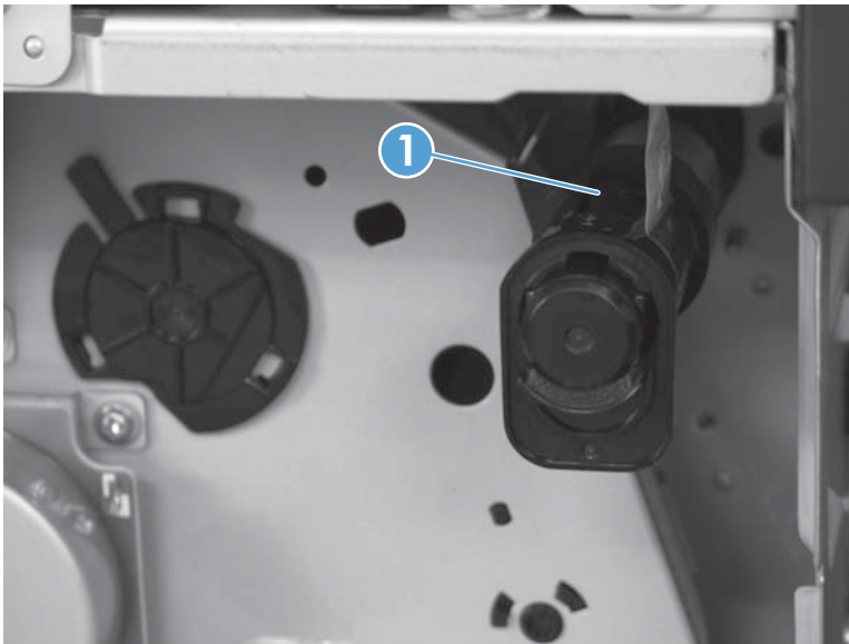
Figure 1-181 Remove the residual toner feed assembly (2 of 6)
