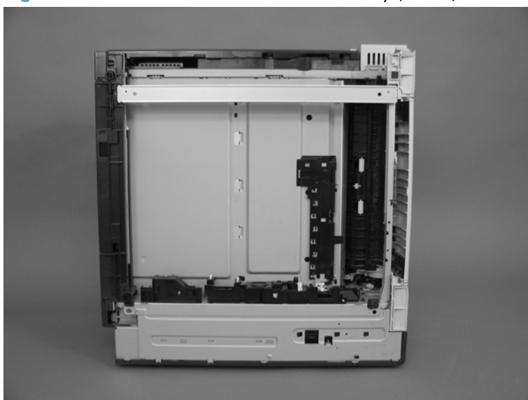
Figure 1-164 Remove the lifter-drive assembly (1 of 3)
