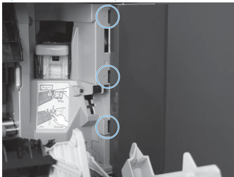
Figure 1-105 Remove the stapler/stacker rear cover (2 of 3)
