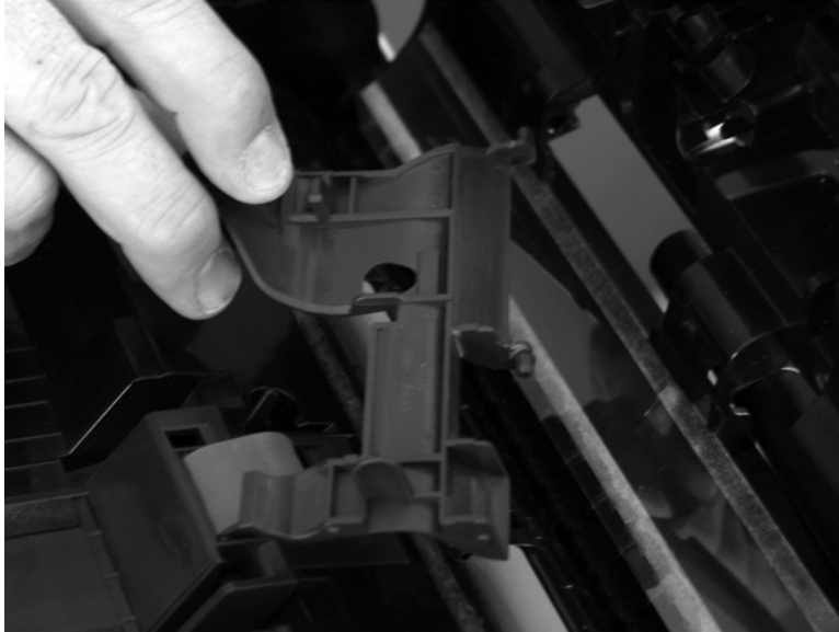
Figure 1-69 Remove the document feeder roller cover (4 of 4)
