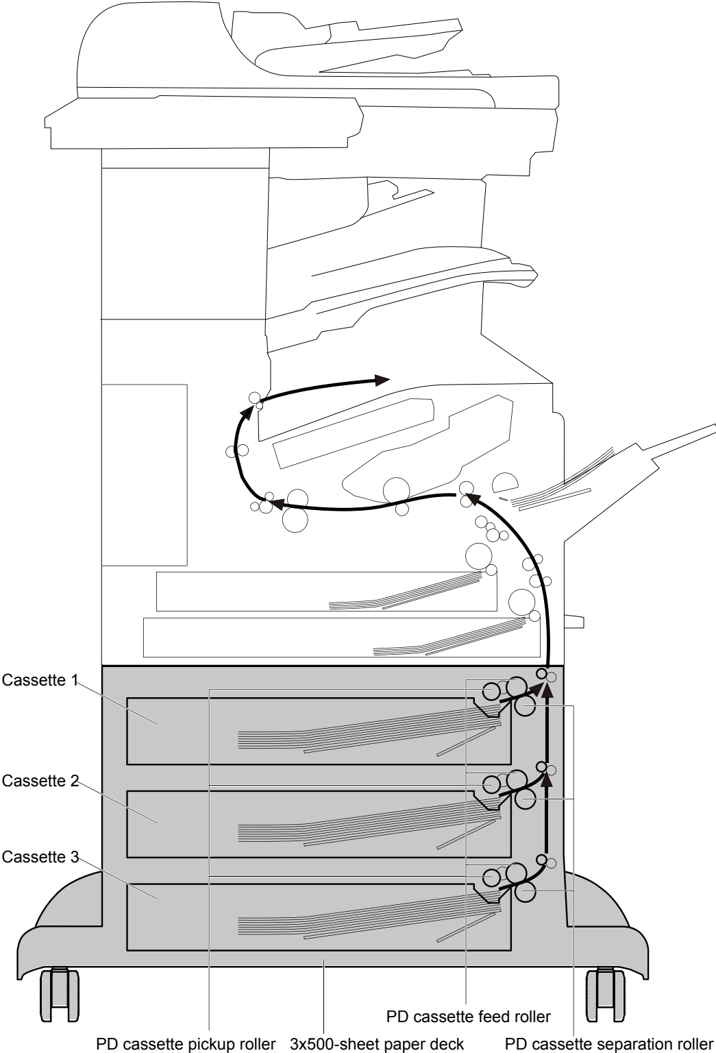
Figure 1-48 Paper deck paper path
