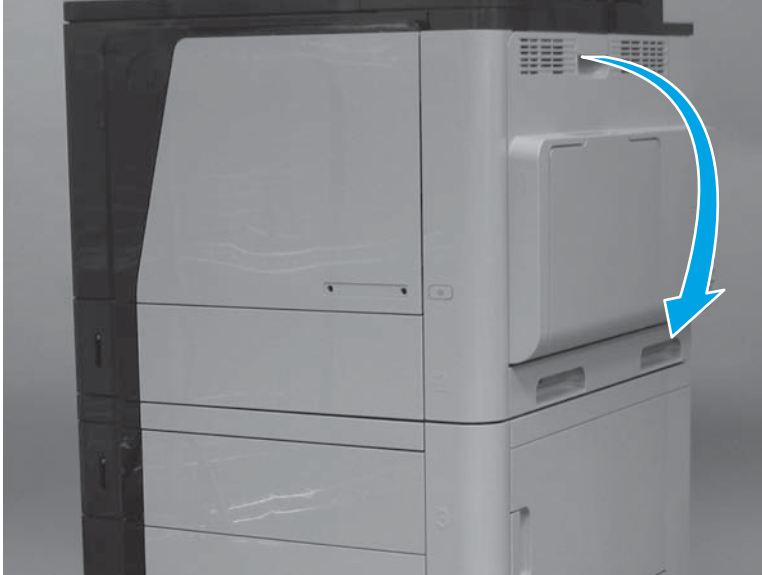
Figure 1-236 Remove the secondary transfer assembly (1 of 3)
