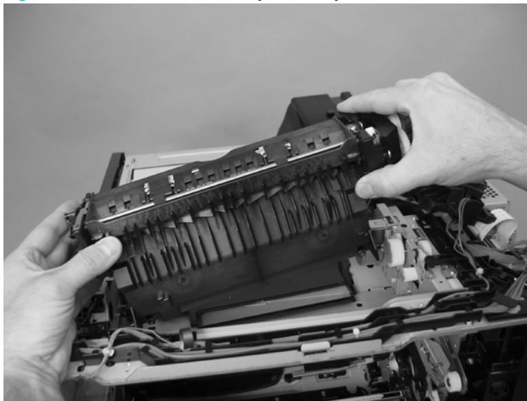
Figure 1-286 Remove the delivery assembly (M651; 7 of 7)
