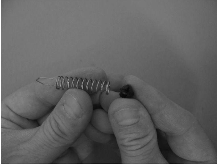
Figure 1-336 Reinstall the lifter base assembly (1 of 2)
