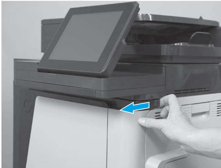
Figure 1-177 Remove the scissor hinge assemblies (1 of 4)
