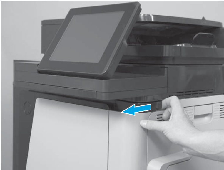
Figure 1-149 Remove the SCB (7 of 13)
