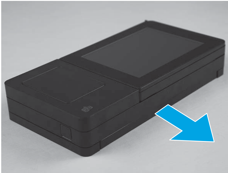
Figure 1-55 Remove the keyboard assembly (M680z; 5 of 7)
