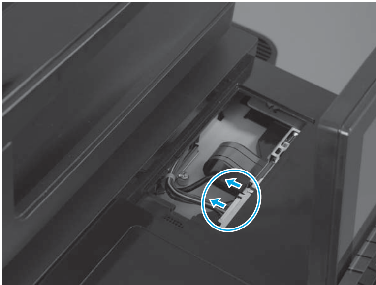
Figure 1-44 Remove the control-panel assembly (M680; 4 of 7)
