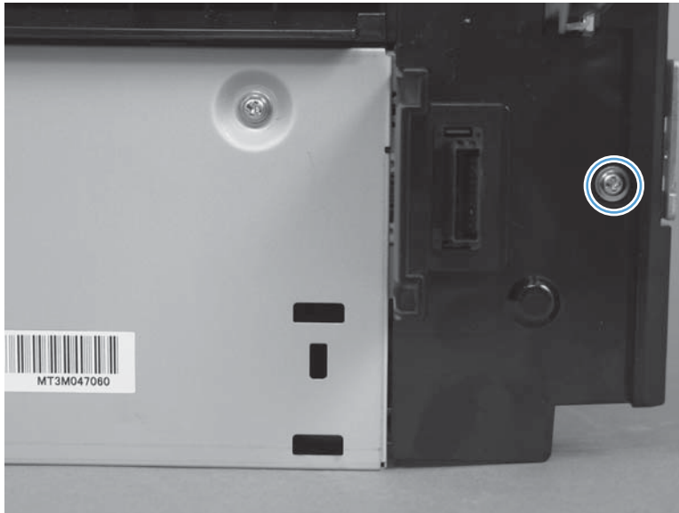
Figure 1-472 Remove the holder connector (stapling mailbox)
