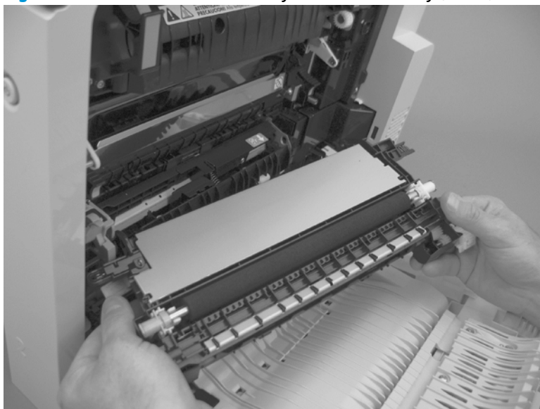
Figure 1-238 Remove the secondary transfer assembly (3 of 3)
