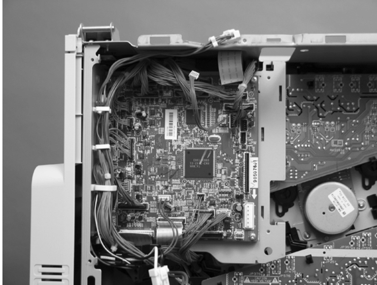
Figure 1-314 Remove the DC controller PCA and tray (1 of 3)
