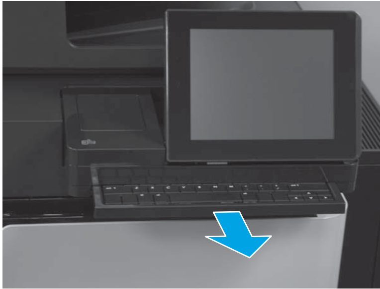
Figure 1-43 Remove the control-panel assembly (M680; 3 of 7)
