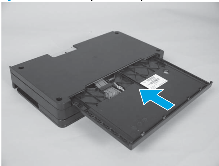
Figure 1-59 Reinstall the keyboard assembly (M680z; 2 of 7)
