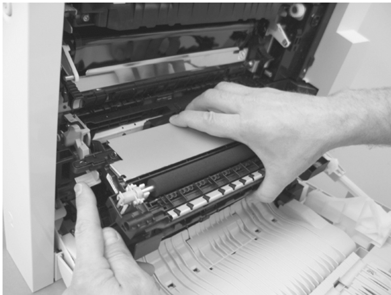
Figure 1-239 Reinstall the secondary transfer assembly
