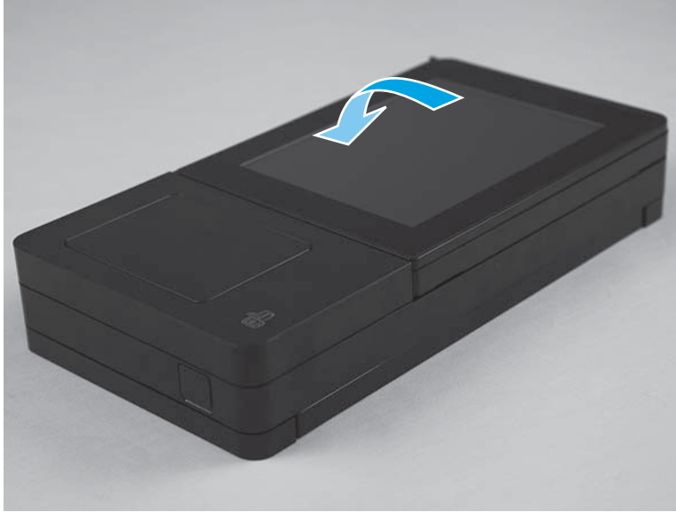
Figure 1-54 Remove the keyboard assembly (M680z; 4 of 7)
