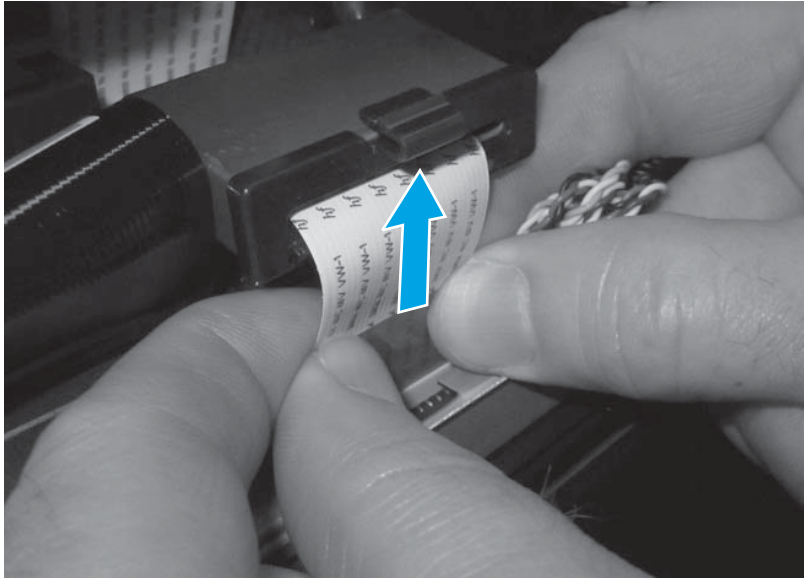
Figure 1-146 Remove the SCB (4 of 13)
