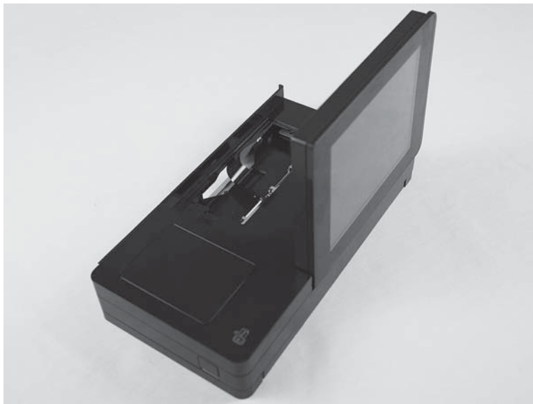
Figure 1-51 Remove the keyboard assembly (M680z; 1 of 7)
