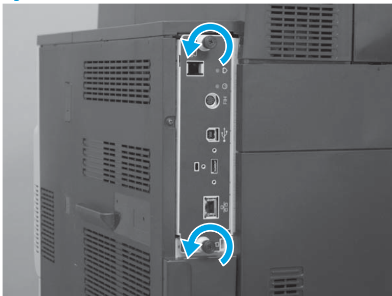
Figure 1-9 Remove the formatter
