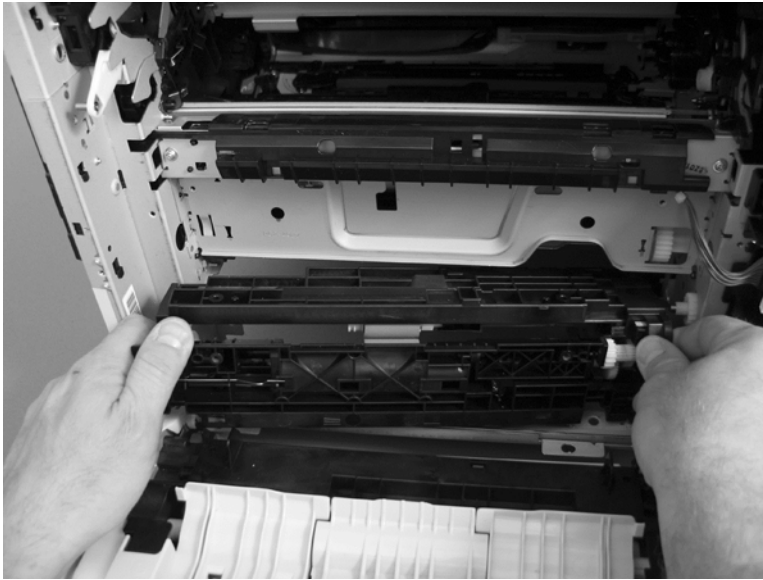
Figure 1-351 Remove the paper-pickup assembly (11 of 11)
