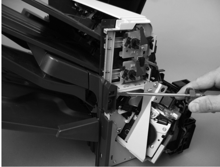
Figure 1-488 Remove the jogger assembly (stapling mailbox; 3 of 3)
