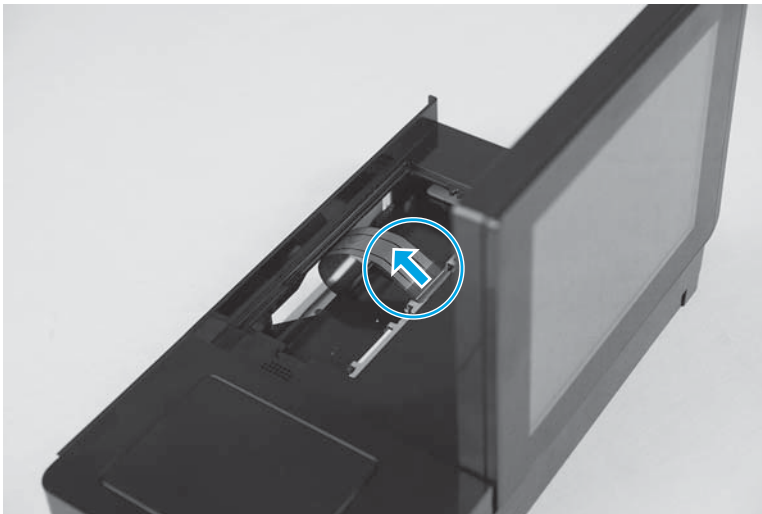
Figure 1-53 Remove the keyboard assembly (M680z; 3 of 7)
