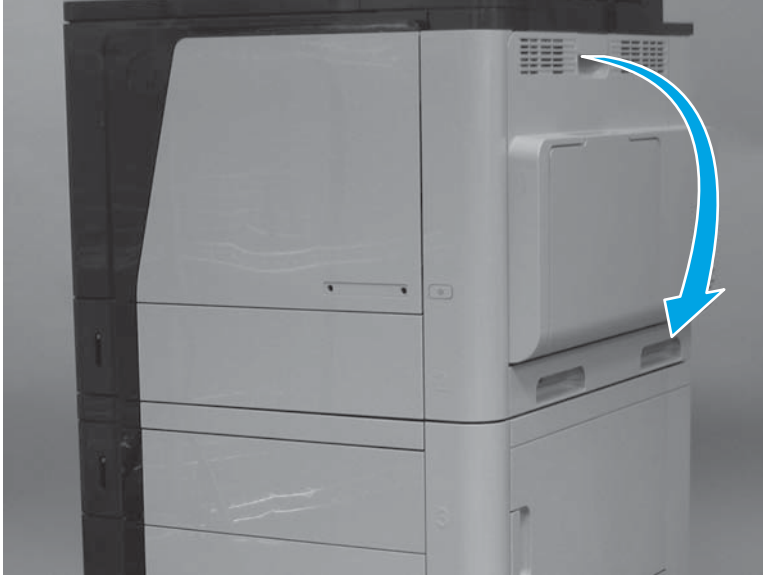
Figure 1-233 Remove the cassette feed guide (1 of 2)
