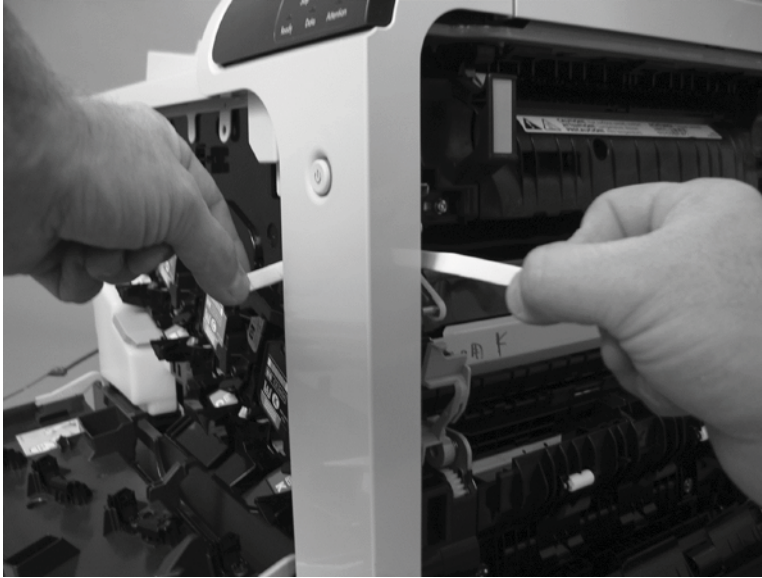
Figure 2-26 Defeating interlocks (2 of 2)
