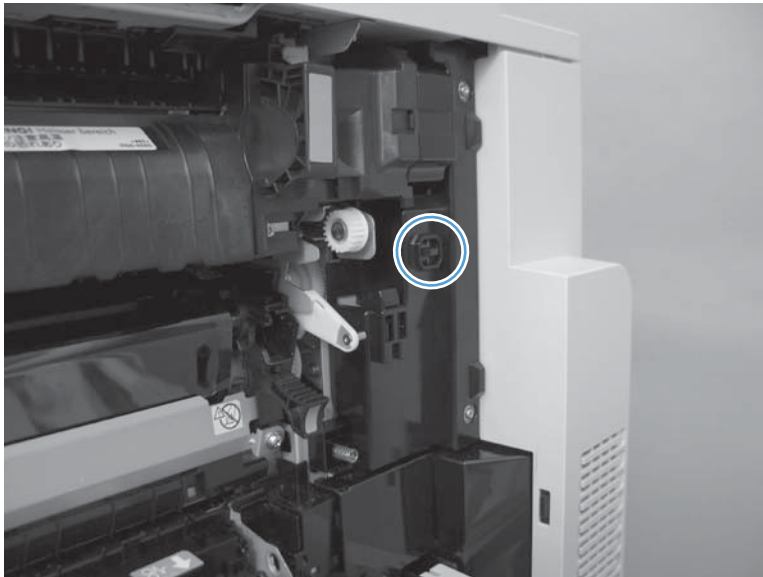
Figure 2-25 Defeating interlocks (1 of 2)
