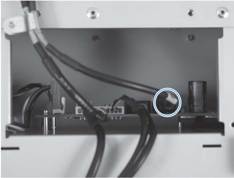
Figure 2-45 Remove the scanner cable (1 of 3)
