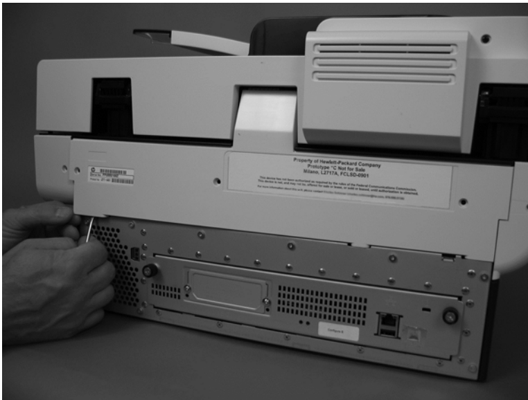
Figure 2-33 Remove the flatbed scanner and ADF assembly (3 of 7)
