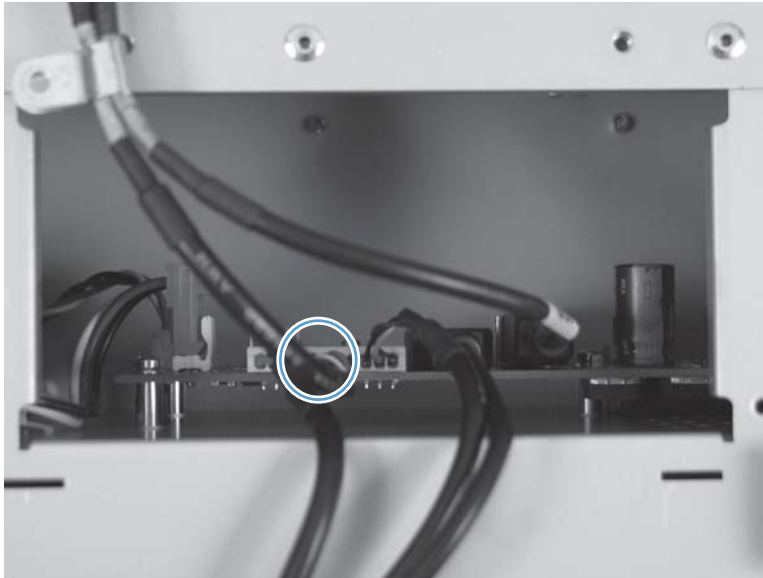
Figure 2-51 Remove the interconnect cable (1 of 4)
