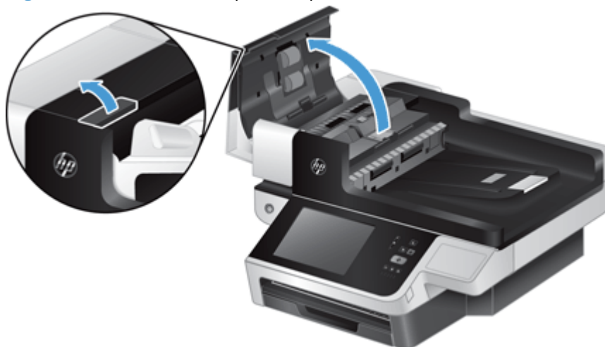
Figure 2-5 Remove the separation pad (1 of 3)
