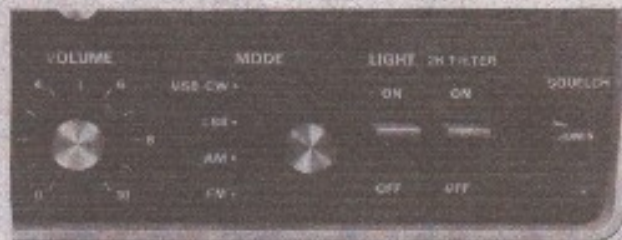
The re-lettered front panel of the FRG-7
